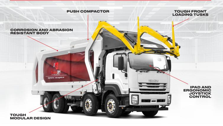
28 M<sup>3</sup> - 33.5 M<sup>3</sup> **BODY CAPACITY HARDOX 450 & BODY MATERIAL HARDOX HIACE STEEL BIN LIFT CAPACITY** 2'500 KG **LOADER POSITION FRONT LOADER** COMPACTOR **PUSH COMPACTOR CONTROL SYSTEM** 12" IPAD INTERFACE **BIN CYCLE TIME 10-12 SECONDS**
